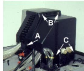
12. Looking into the upper mechanical assembly from the rear of the processor, locate the Diode PC Board.
