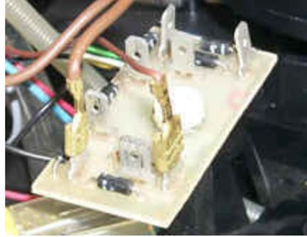
13. If the pumping quantities are *too low*, then move the larger diameter brown wire closer to the narrow brown wire. If the pumping quantities are *too high*, then move the larger diameter brown wire further away from the narrow brown wire.
