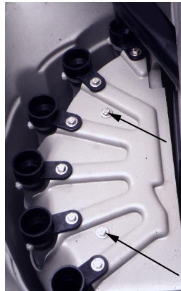
2) Remove the screws that hold the reclamation plate in place.
