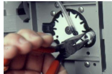
4) Observe the hole in the CAM is D-shaped.
