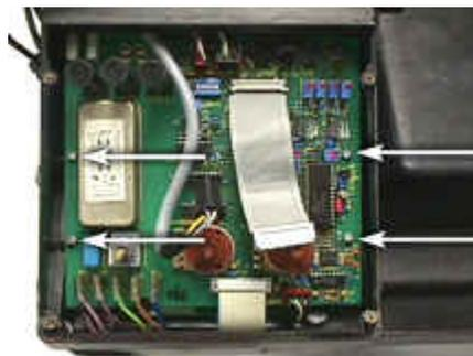
20.2. Locate and remove both the gray colored ribbon cable and the four (4) pin connector near the bottom of the lower interface circuit board.
