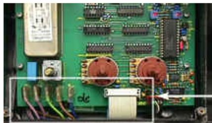
20.4. Locate and remove the two (2) connectors labeled CHE and WA (the labeling is printed on the circuit board) at the upper right-hand side of the lower interface circuit board.
