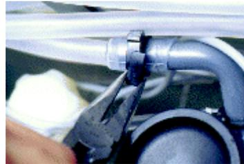
5. Disconnect all of the air lines from the bottles, keeping the black plastic 90° angle elbows attached to the hoses.
