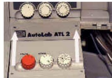
11. Pull the access panel forward being careful not to lose the rubber grommet located on the right side of the panel.
