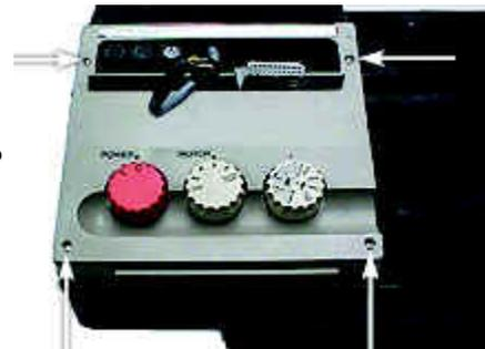
16. Remove the three switch knobs by pulling them upward.
