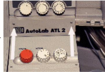
7) Pull the access panel forward being careful not to lose the rubber grommet(s) located on the right side of the panel.
