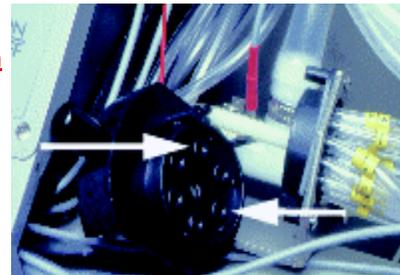
**DO NOT** remove the air hoses from the top half of the front/back bottle (air) switch!
