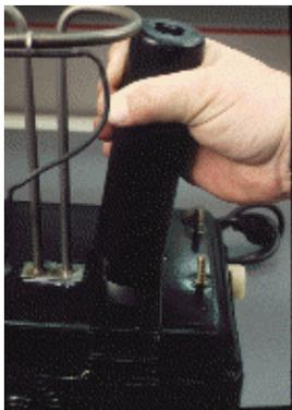
1. Turn the unit upside down and remove the pump housing from its receptacle, using a rocking motion, and pull it away from the motor unit.
